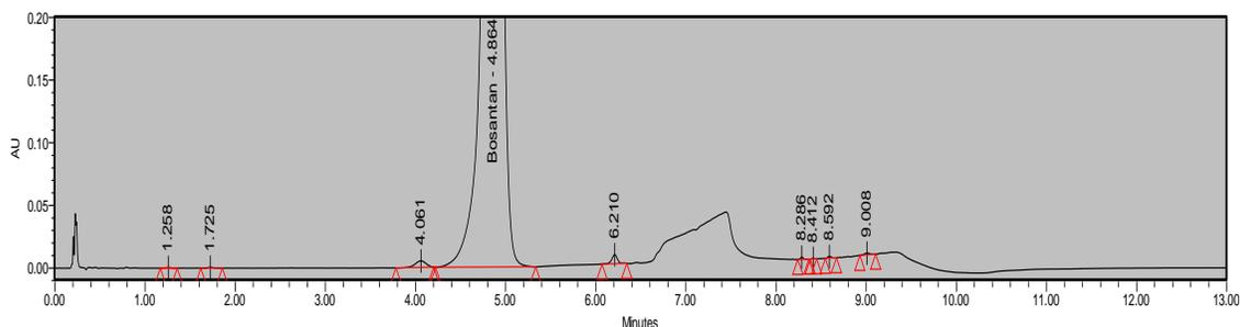
**Figure 5: Acid degraded sample chromatogram**
