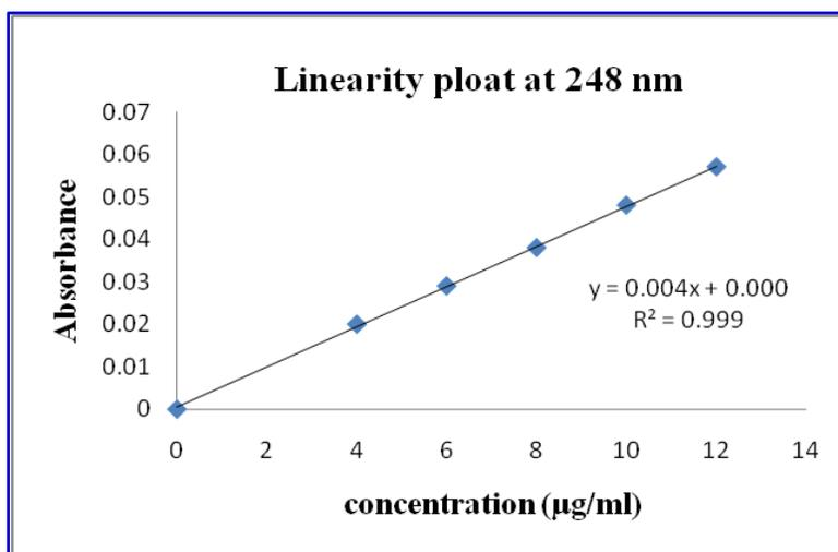
Figure 5. Calibration curve for Iloperidone at 248nm by Second order derivative spectroscopy
