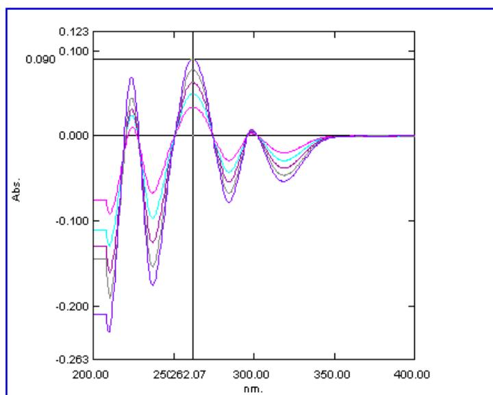
**Figure 2: Overlay first order derivative spectra of Iloperidone showing absorbance at 262nm**
