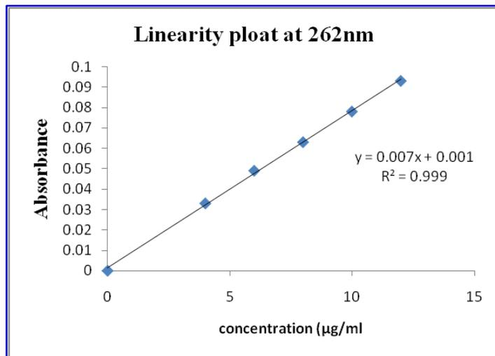
Figure 3. Calibration curve for Iloperidone at 262nm by 1<sup>st</sup> order derivative spectroscopy
